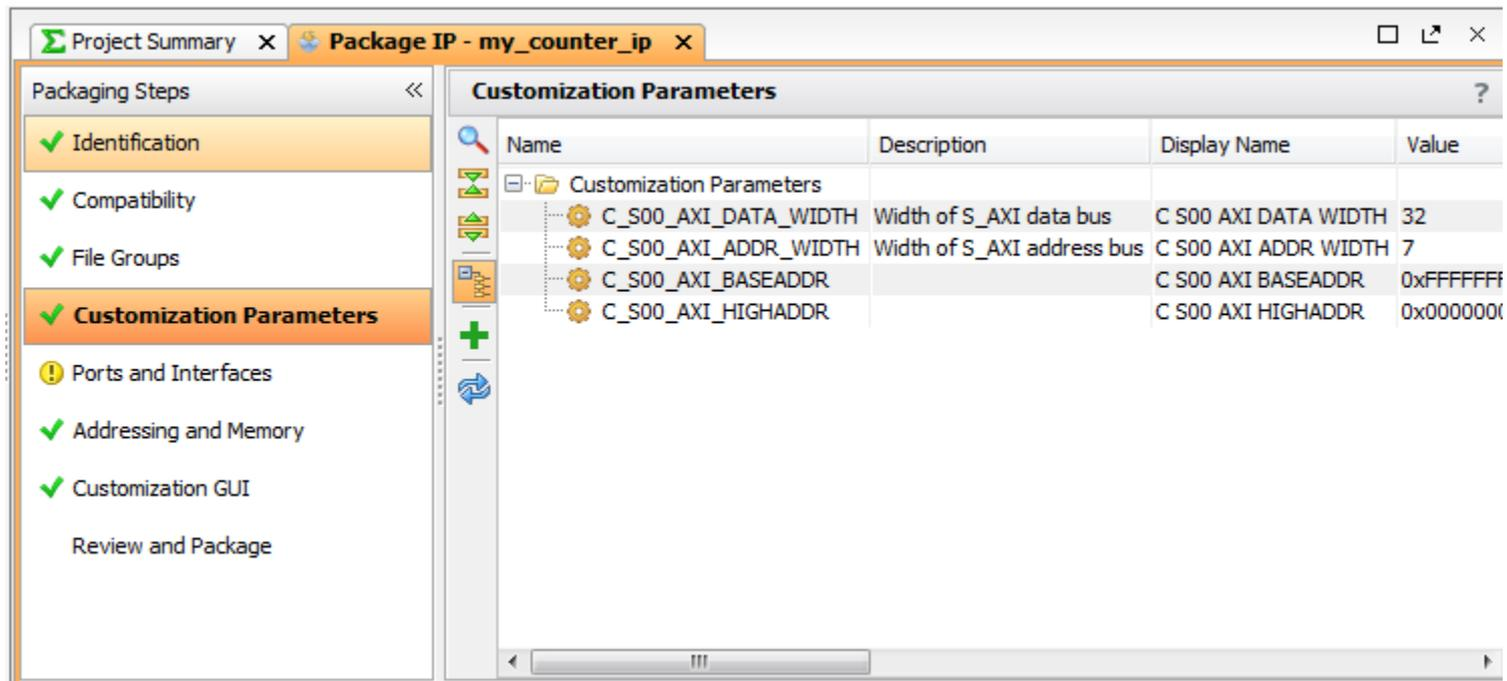
The screenshot shows the Xilinx Vivado interface with the 'Customization Parameters' window open. The 'Packaging Steps' sidebar on the left has 'Customization Parameters' selected. The main window displays a table of parameters:
